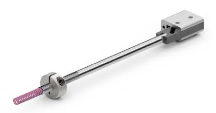
Mini Sliding Lifters are a new generation undercut release system. They offer innovative options for mould designers. Integrated Cam tracking system makes use of the part undercut itself to move forward supported by the spring underneath.
